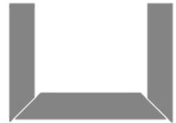
Apply [Wood Glue](#) to the exposed miter cut grain of the two bottom corners. Fasten the screws into the countersunk holes. The force of the screw will then pull the corners flush.
