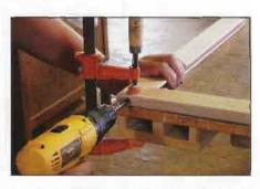
When drilling the holes, put the countersink hole on the height of your piece. Therefore, by the screws going into the side, the weight sits on the length of the screw and is not pulling on the thread. If you are not using a countersink, you can use brass-plated framing screws to accent the look of your frame by drilling a 7/64" pilot hole and inserting the screw. Drill all four sides before trying to insert the glass.
