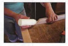
For solid, accurate corners, use the glue/screw technique. Beginning with the bottom and sides of the frame, apply woodworking glue to the exposed sides of the miter and then lay them on the table "assembled." If you plan on adding a finish or stain, be careful to not let the glue squeeze out onto the face of the frame. The glue may mar the appearance after it is applied.
