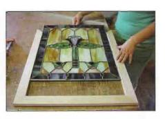
After you have assembled the three sides, slide your glass into the "U" shape. By not gluing the upper corners, you will allow for later disassembly.
