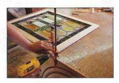
For the best results, use a clamp to keep the screw holes aligned. A helpful hint for making sure that your corners line up properly is to place the countersink corner about 1/16" to 1/8" over the pilot hole corner. The force of the screw will then pull your corners flush.
